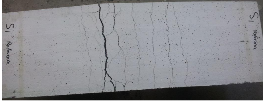
Figure 34: Crack pattern of control slab S1 (without strengthening)
