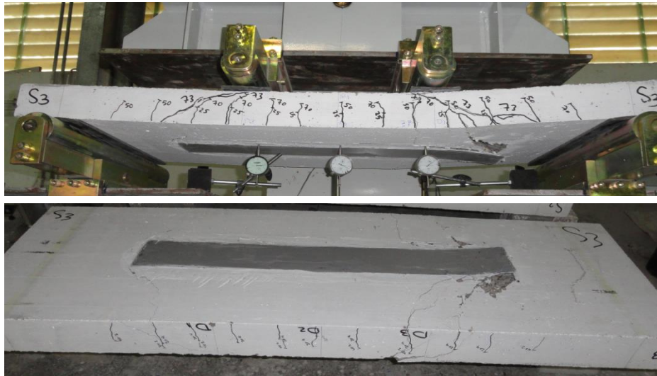
Figure 36: Crack pattern of strengthening slab S3
